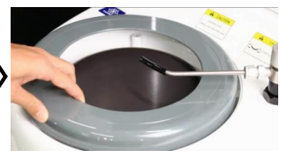
Platen replacement & sample placement 50s
